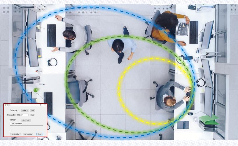
Set presence detection zones based on distance from sensor.
