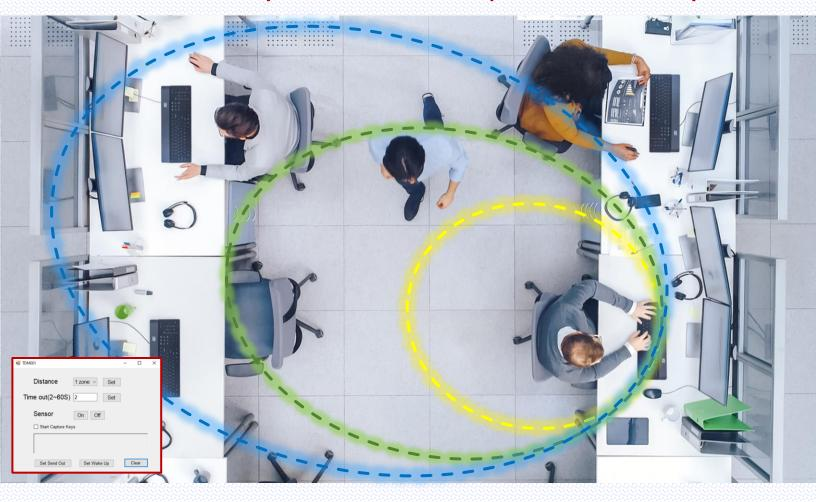
Set detection zones based on distance from sensor
