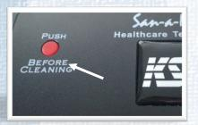
**Step 1** — PUSH the easy-clean red LinkSmart<sup>™</sup> button once to disengage keys. The keys lock, and the Num lock, Caps lock and Scroll lock LED's flash simultaneously, indicating the keyboard is in cleaning mode. You are now able to wipe the surface without risk of entering errant data.
