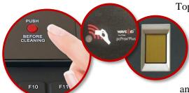
Top Strip integration of RFIDeas<sup>®</sup> dual band card reader makes contactless "tap-in, tap-out" logon-logoff fast and easy. When combined with an embedded silicon-surfaced pro-grade 500dpi Crossmatch<sup>™</sup> fingerprint sensor, customers are ensured irrefutable dual authentication that is <u>ePrescribe</u> and <u>FIPS 201</u> compliant. The RFIDeas<sup>®</sup> card reader and Crossmatch<sup>™</sup> sensor are fully compatible with leading SSO and EMR applications.
